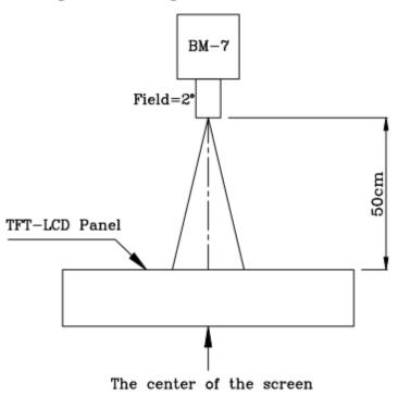
**②The Brightness Test Point Setup**
