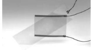
can fracture glass. The solution is a clear heating element that can provide heat to the entire surface.
