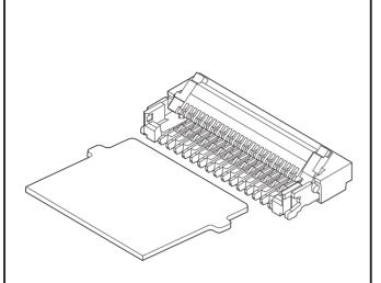
0.2mm pitch FVX connector for FPC has been developed for small portable equipment for which low profile and miniaturization are required. By using FPC with protrusions, the positioning accuracy of FPC is improved.
