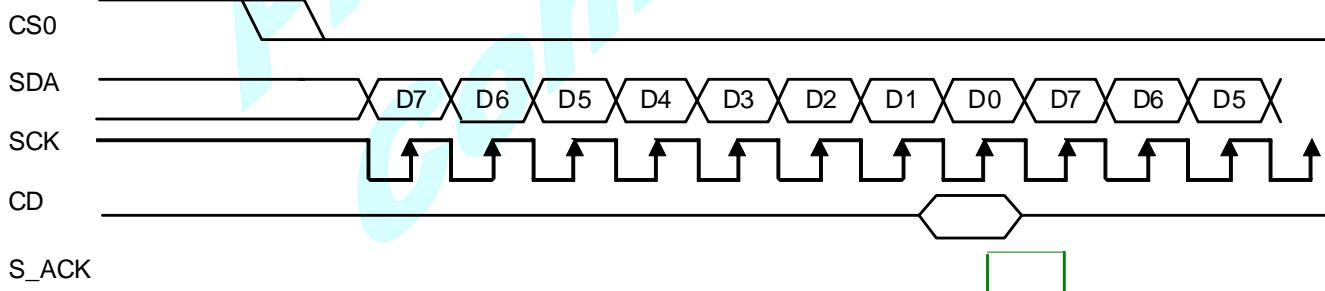
FIGURE 4.b: 4-wire Serial Interface (S8) – Write
