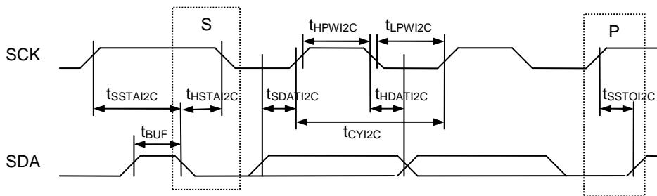
FIGURE 20: Serial Bus Timing Characteristics (for I<sup>2</sup>C)
