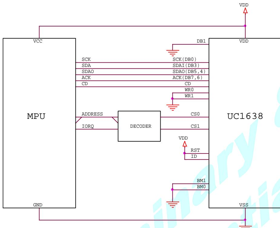
FIGURE 9: 4-Wire SPI (S8) serial mode reference circuit
