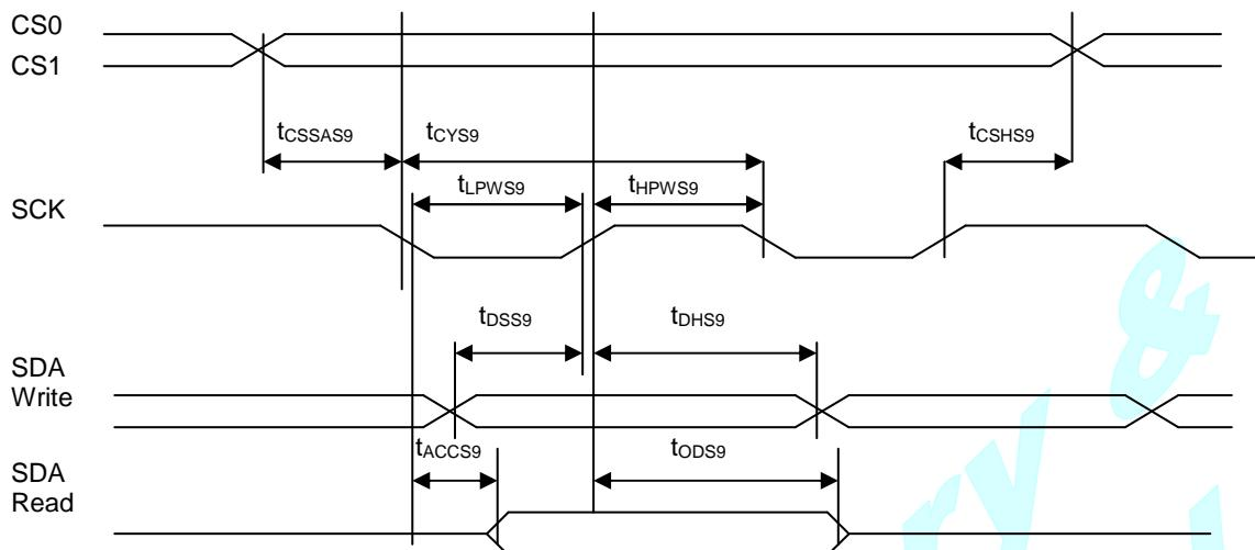
FIGURE 19: Serial Bus Timing Characteristics (for S9)
