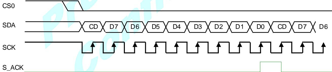
**FIGURE 5.b:** 3-wire Serial Interface (S9) – Write
