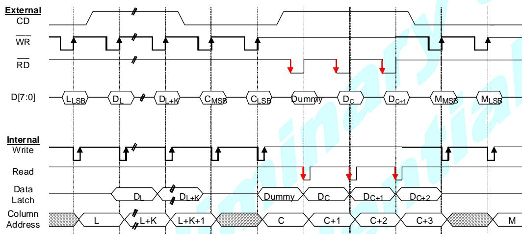
FIGURE 3: 8-bit Parallel Interface & Related Internal Signals
