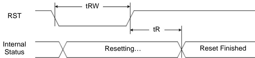
FIGURE 21: Reset Characteristics
