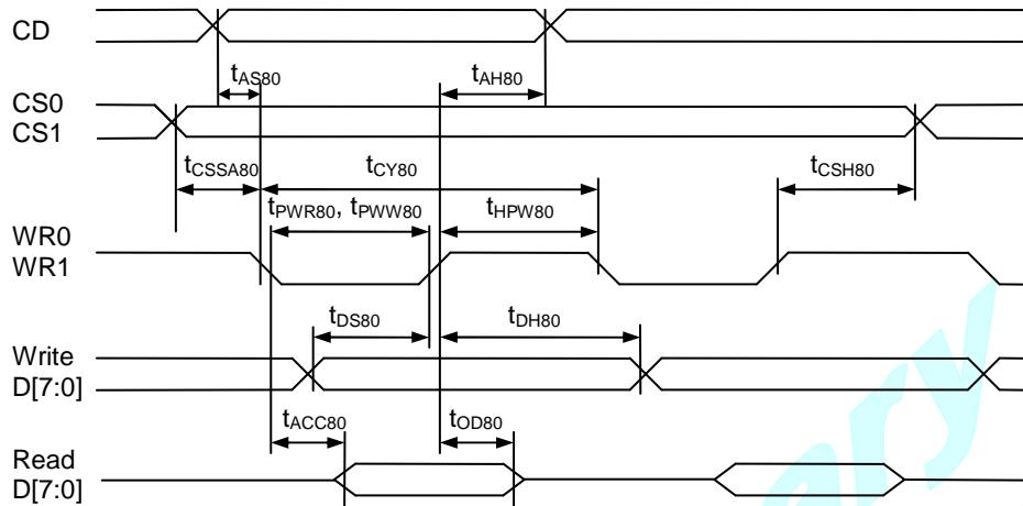
FIGURE 16: Parallel Bus Timing Characteristics (for 8080 MCU)
