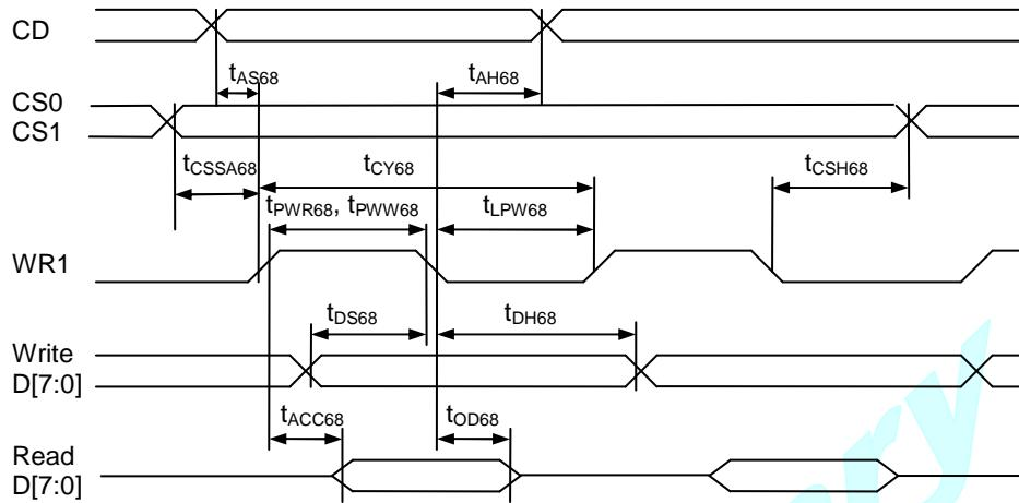
FIGURE 17: Parallel Bus Timing Characteristics (for 6800 MCU)
