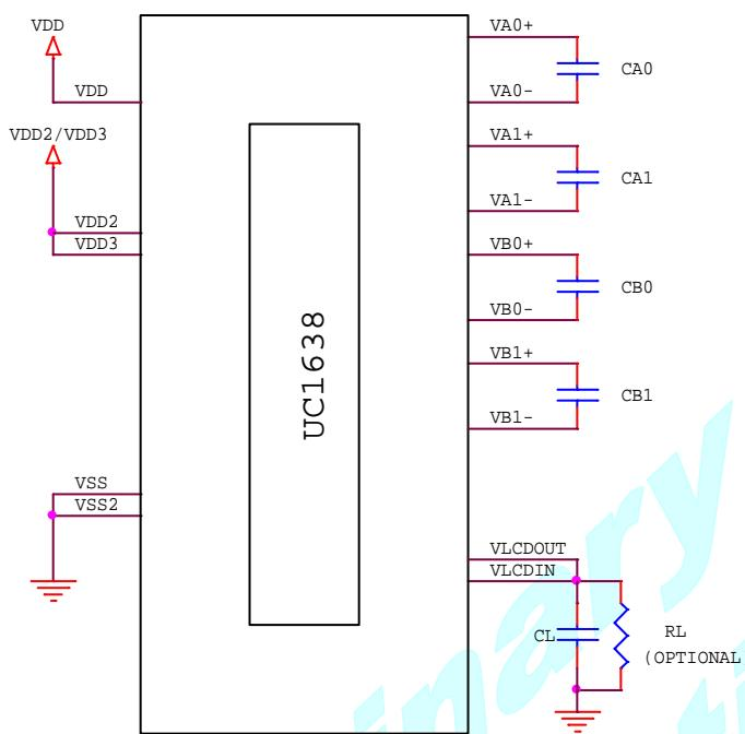
**FIGURE 1.a:** Reference circuit using INTERNAL Hi-V generator circuit
