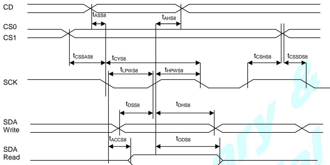
FIGURE 18: Serial Bus Timing Characteristics (for S8)
