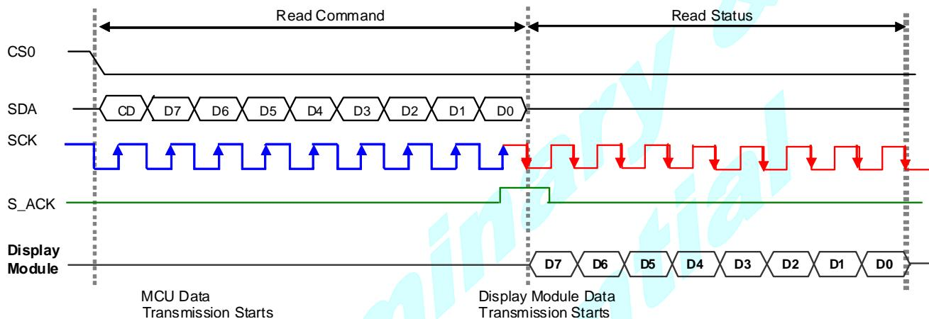
**FIGURE 5.a:** 3-wire Serial Interface (S9) – Read
