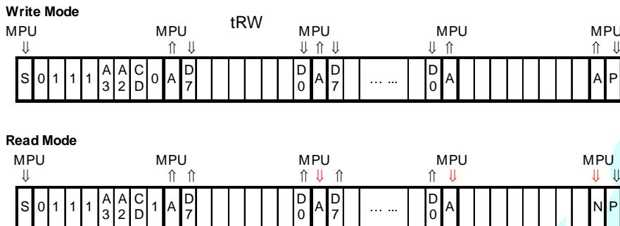
**FIGURE 6: 2-wire Serial Interface (I<sup>2</sup>C)**
