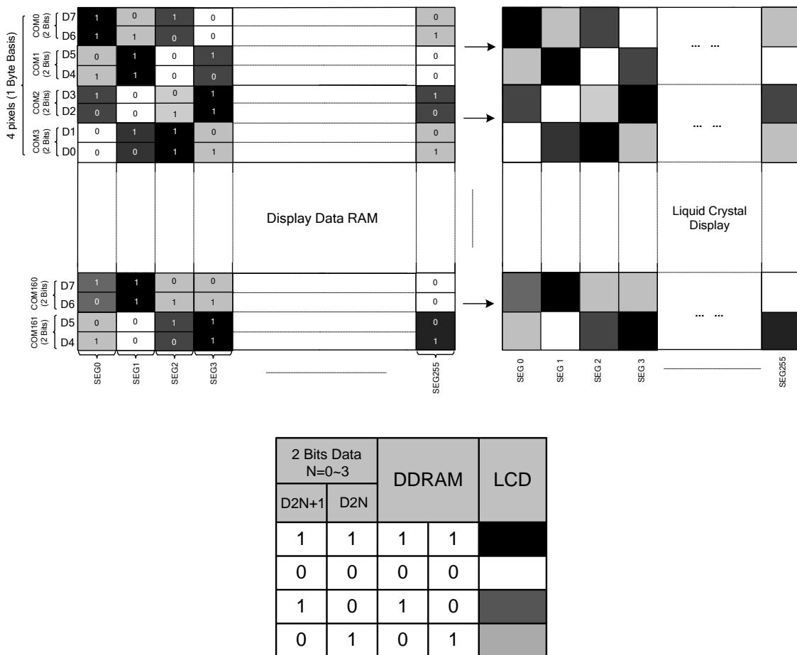
Figure 21 DDRAM Mapping (4-Level Gray Scale Mode)
