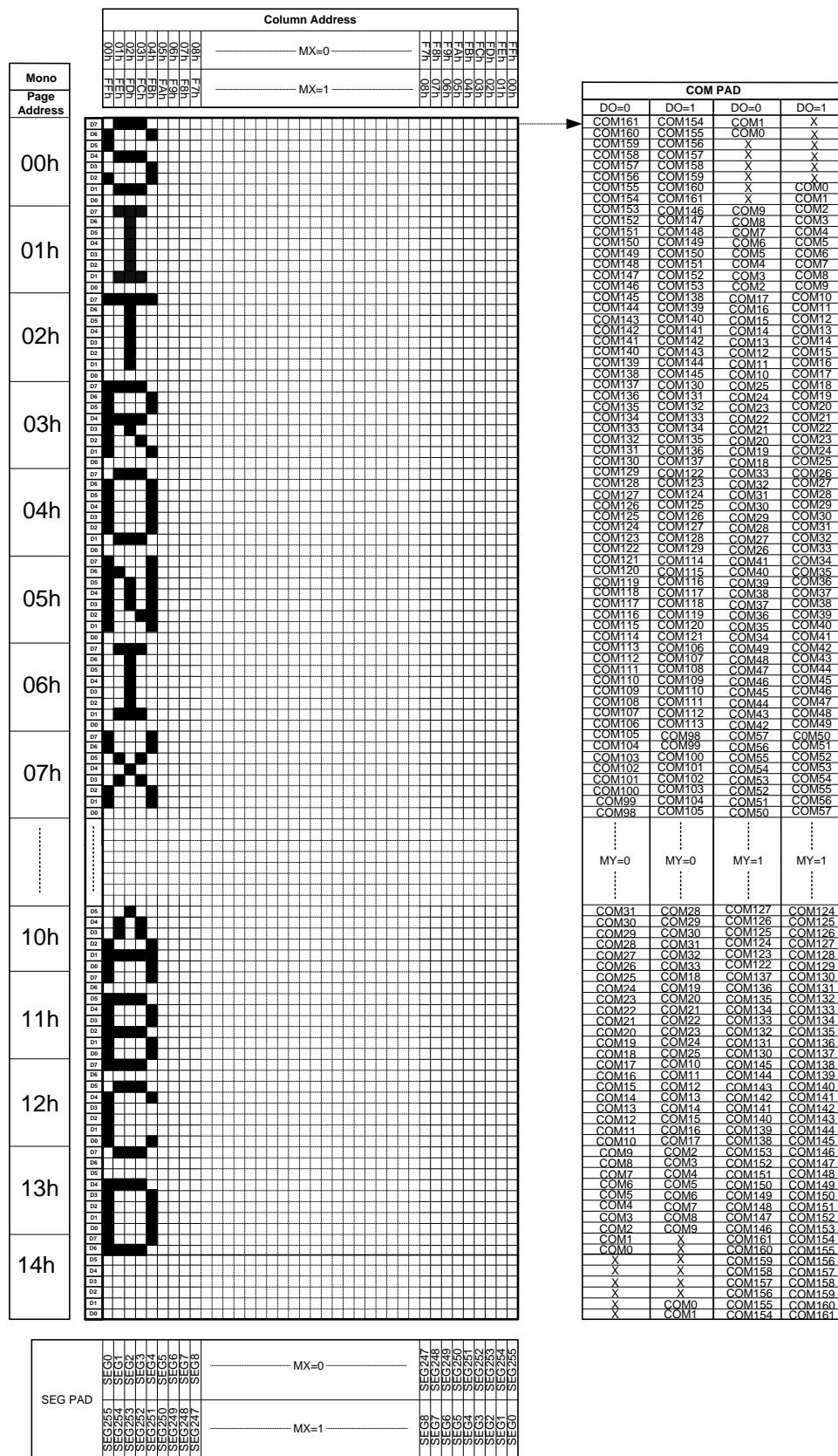
**Figure 29 DDRAM Display Direction (Monochrome Mode; COMSCN=1)**
