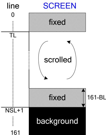
TL[7:0] is to specify the top line address of the scrolled + background areas. Specify the 0th line for the top screen scroll or whole screen scroll.
