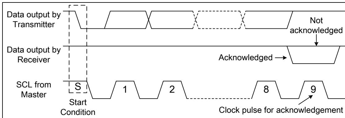
**Figure 17 Acknowledgement of I<sup>2</sup>C Interface**
