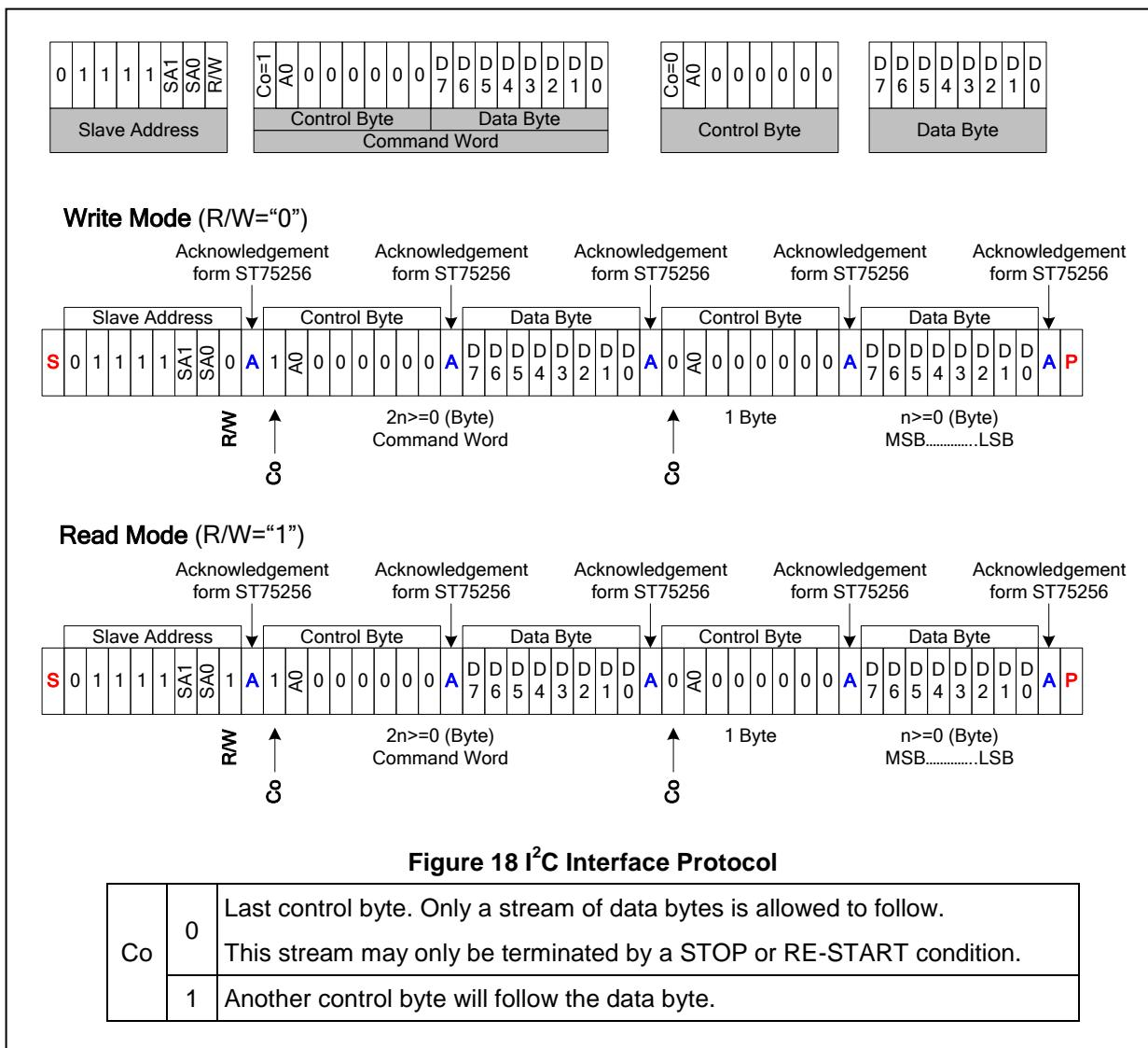
Figure 18 I<sup>2</sup>C Interface Protocol
