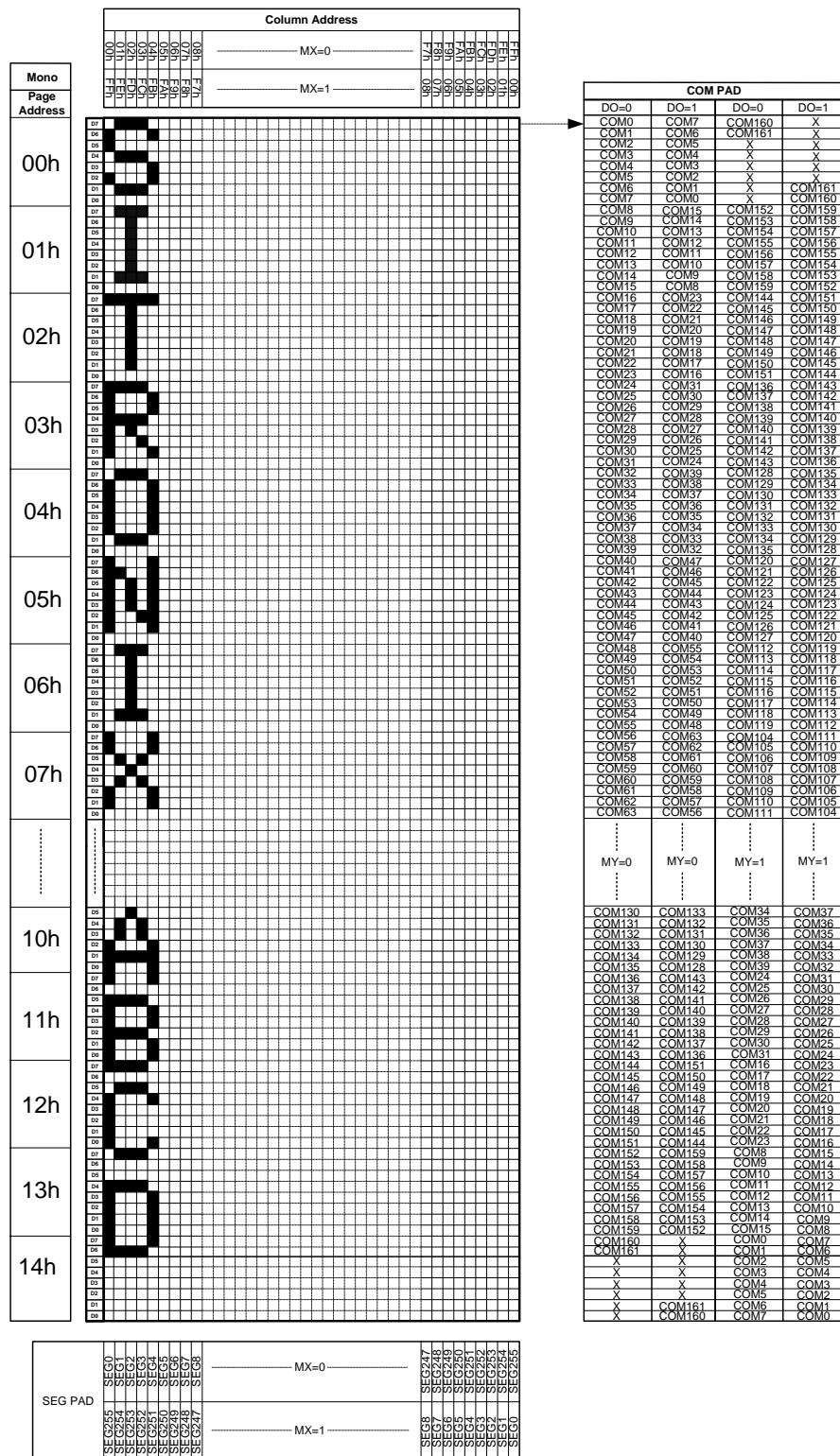
Figure 27 DDRAM Display Direction (Monochrome Mode; COMSCN=0)
