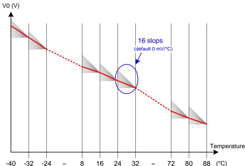
**Figure 40 Temperature Compensation Coefficient Selection**
