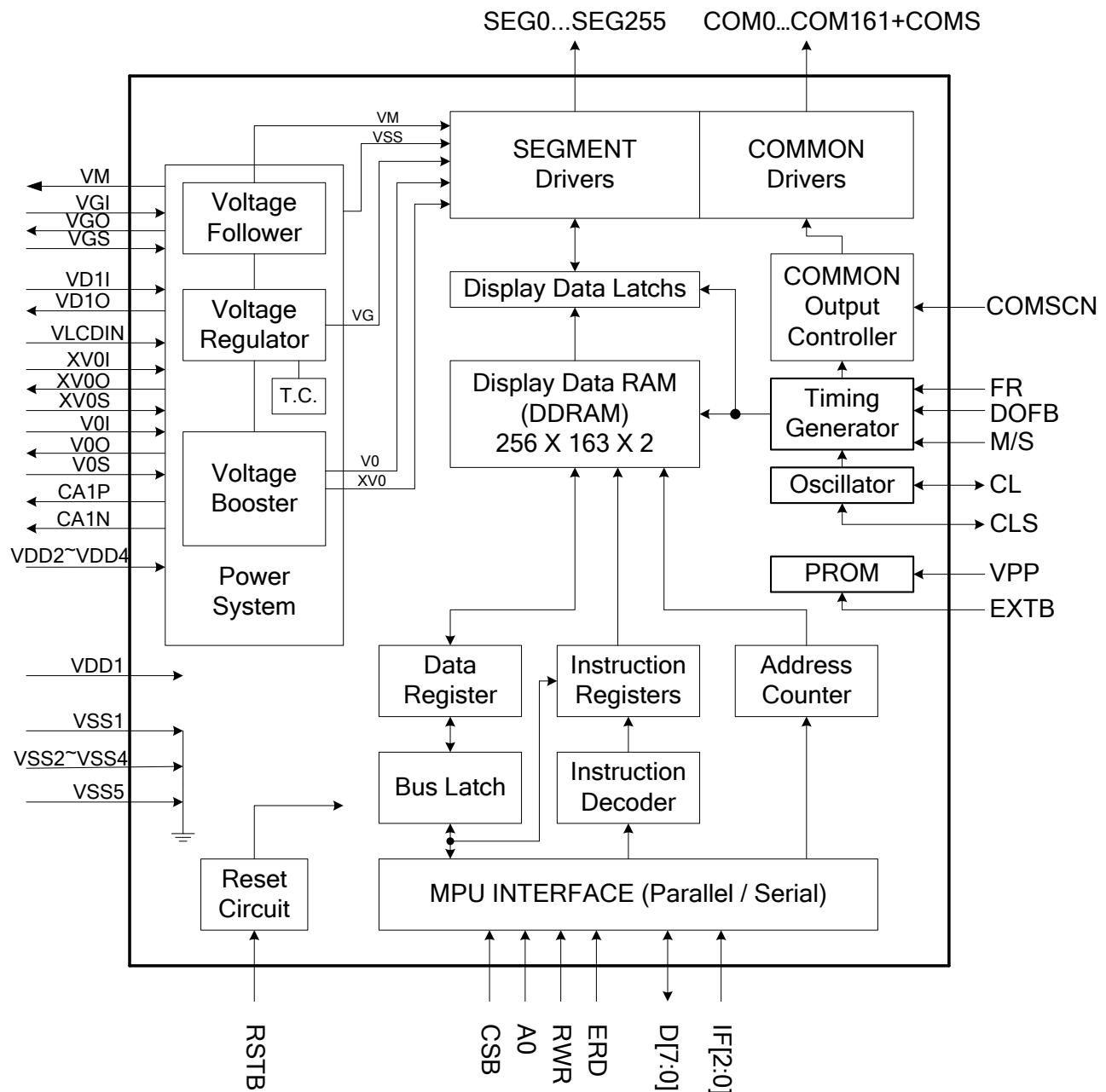
Figure 2 Block Diagram
