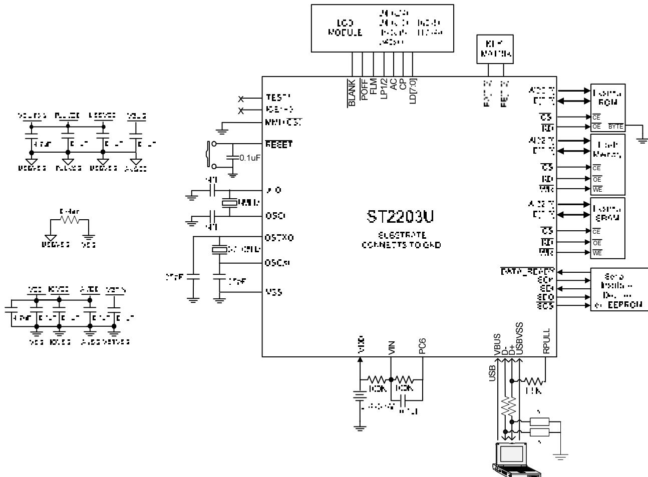
When using internal regulator output as system power, the application is shown below:
