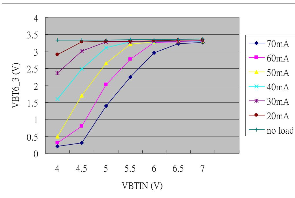
VBTIN is the input of the regulator, and VBT6\_3 is the output. One should notice the loading capability when using internal regulator.
