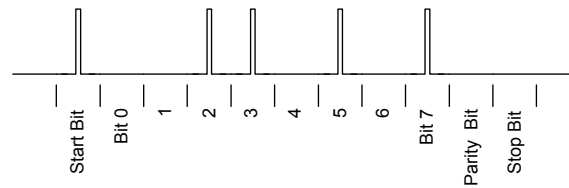
FIGURE 18-3 IrDA ASCII "S" with Odd Parity
