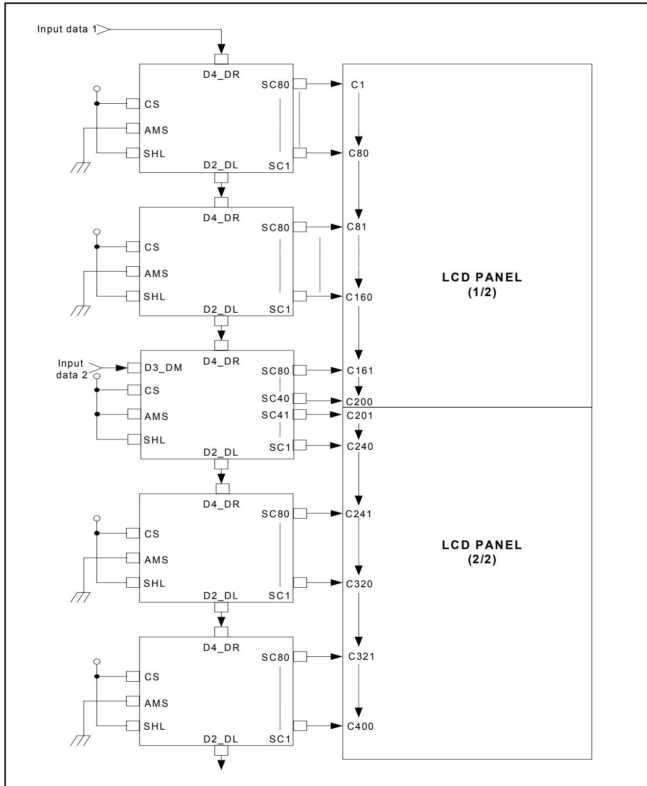
**Note:** Using this application mode (dual-type common mode), the duty ratio can be reduced to half. In case, 1/200 duty can be used to drive the 400 common LCD panel.
