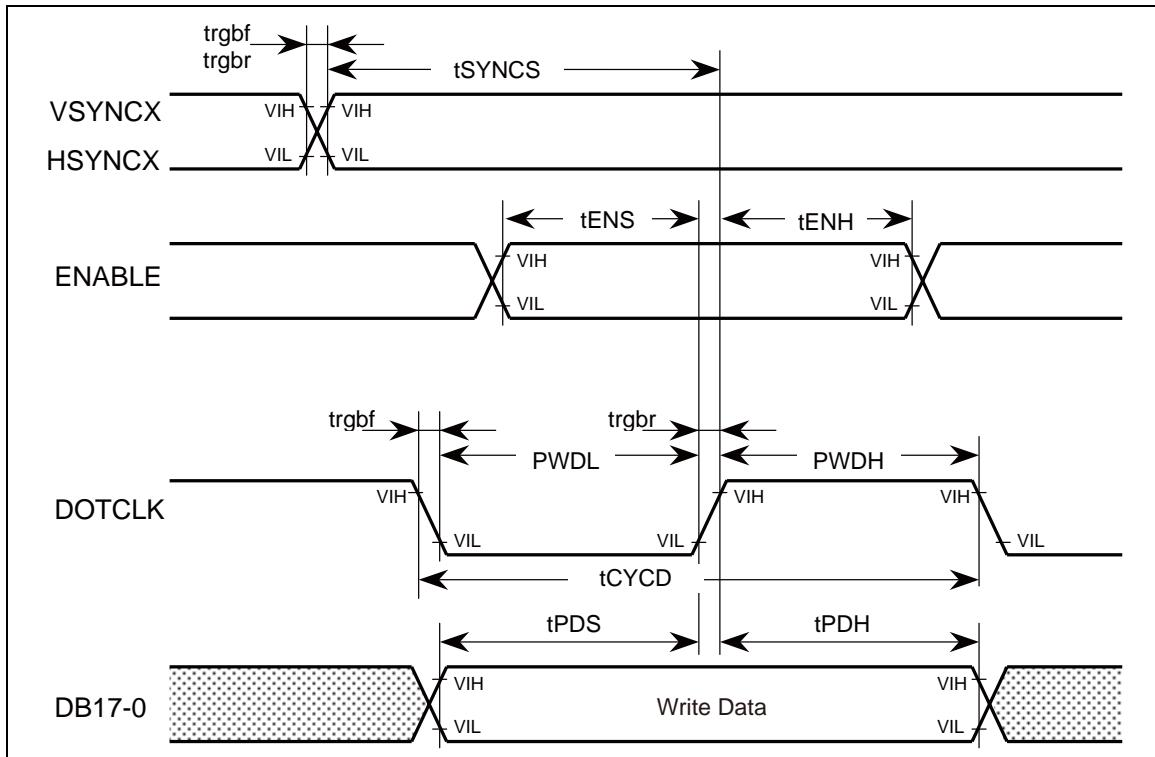
**Figure D RGB Interface Timing****LCD Driver and VCOM Output Characteristics**
