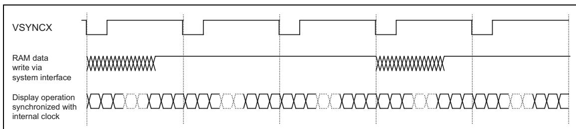
**Figure 34** Moving Picture Data Transfers via VSYNC Interface
