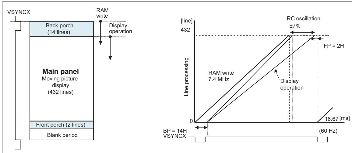
Figure 35 Write/Display Operation Timing via VSYNC Interface
