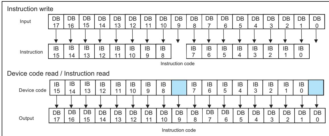
**Figure 15 18-bit Interface Data Format (Instruction Write / Device Code Read / Instruction Read)**
