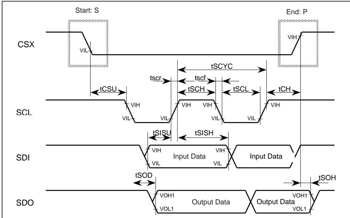
**Figure B Clock Synchronous Serial Interface Timing****Reset Operation**
