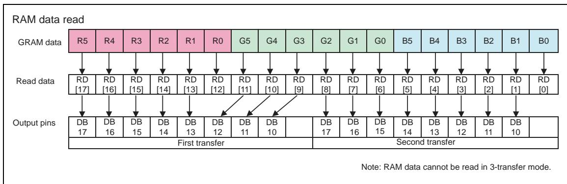
**Figure 29** 8-bit Interface Data Format (RAM Data Read)
