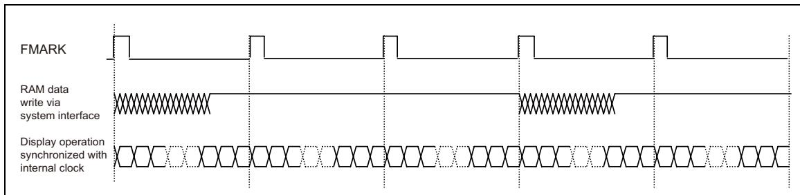
**Figure 39 Moving Picture Data Transfers via FMARK Function**
