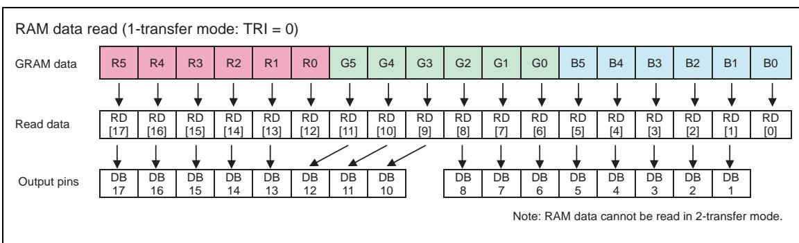
Figure 20 16-bit Interface Data Format (RAM Data Read)
