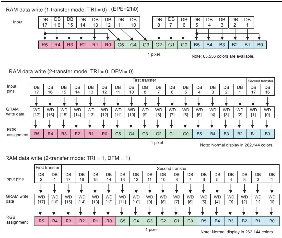
Figure 19 16-bit Interface Data Format (RAM Data Write)
