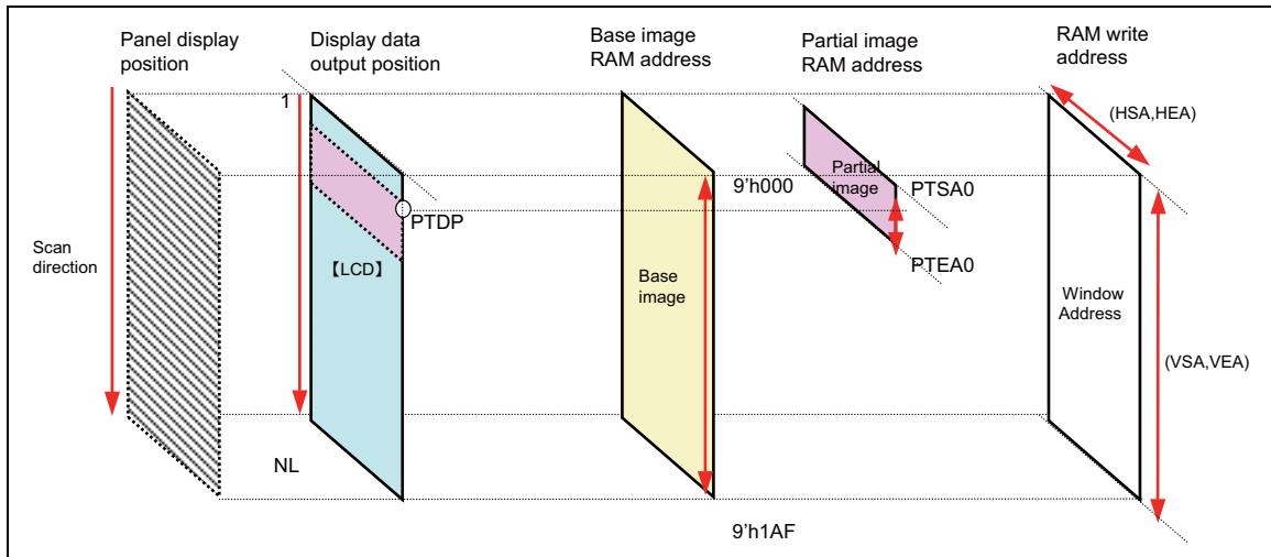
Figure 50 RAM Address, Display Position and Drive Position
