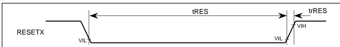
**Figure C Reset Timing**
