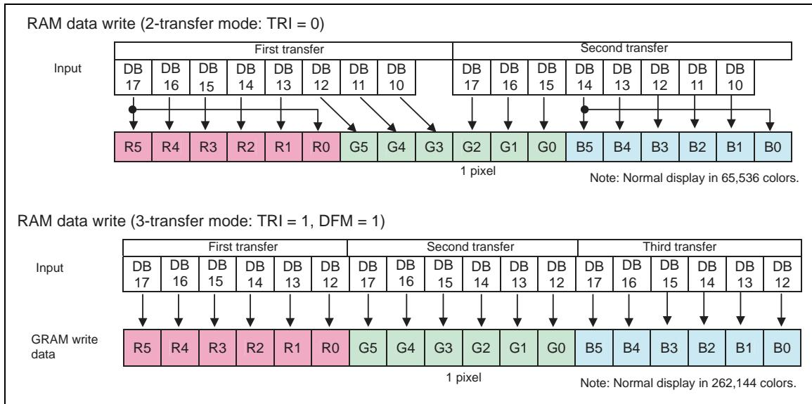
**Figure 28 8-bit Interface Data Format (RAM Data Write)**
