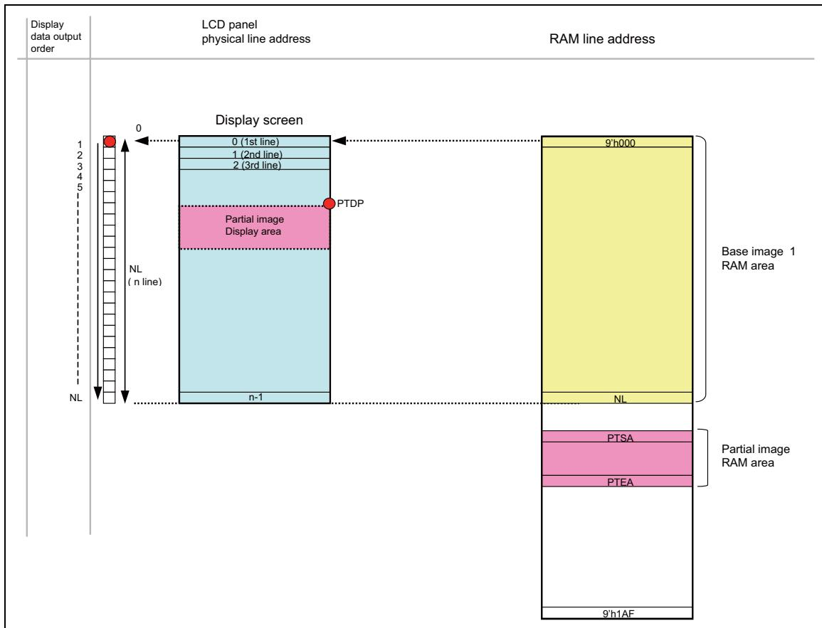
**Figure 51 Display RAM Address and Panel Display Position**
