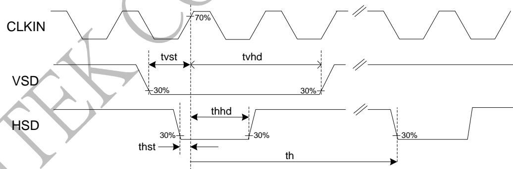
Source output timing diagram
