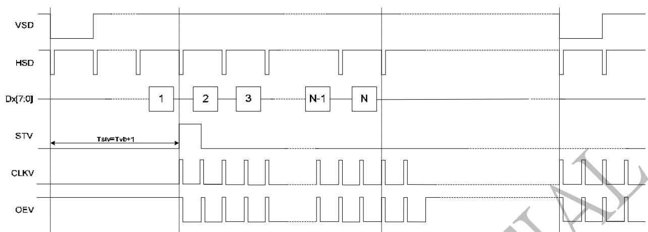
Vertical Timing Diagram of DE Mode (Dual Gate)
