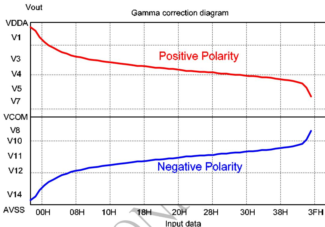
Note: AVDD-1 > V1 > V3 > V4 > V5 > V7; V8 > V10 > V11 > V12 > V14 > AGND+0.1V
