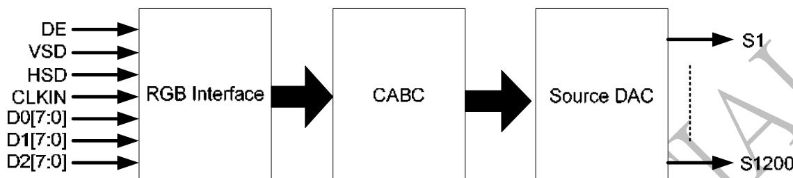
The CABC function can be turned ON/OFF via external pin as CABC\_EN and also can be configured by software commands via SPI mode for performance optimization. ILI6123 can calculate the backlight brightness level and send a PWM pulse to LED driver via CABC\_EN pin for backlight brightness control purpose. The figure in the following is the basic timing diagram which is applied ILI6123 to control LED driver.
