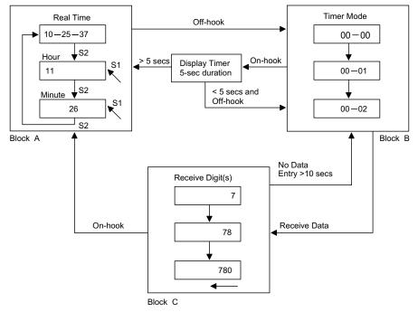
Note: Block A shows the switches S1 and S2 that are used for setting and selecting. Block B illustrates a timer mode when Off-hook; timer resets and starts to count the conversation time. Block C displays blinking "—". After Off-hook, dialing data is received and displayed on the LCD from left to right. When the entry interval is over 10 seconds, the timer resets and starts to count.
