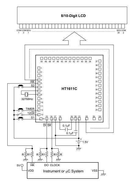
\* The IC substrate should be connected to VDD in the PCB layout artwork.
