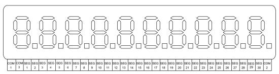
LCD driving system 1/2 bias, 1/3 duty, 3V
