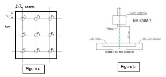
FIG.3. The definition of viewing angle
