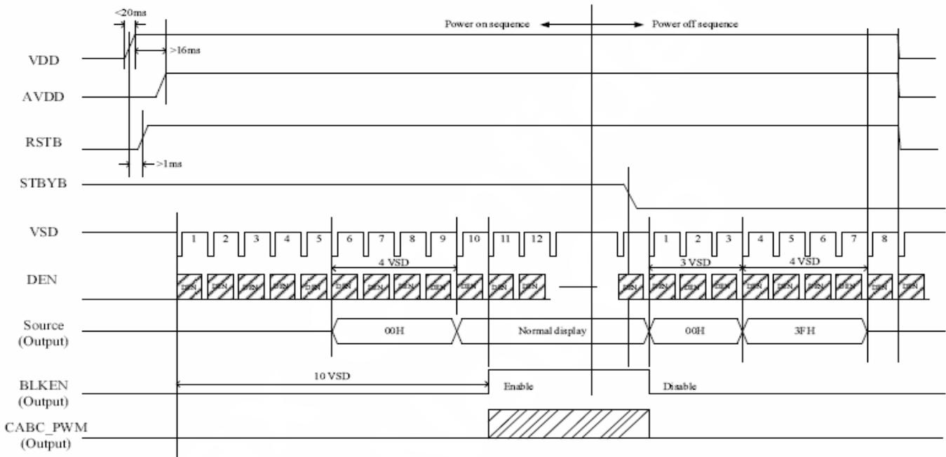
To prevent device latch up or power on display noise, the power on/off sequence shown below must be followed. After VDD reaches 1.8V, VGH/VGL can start to power on. Before VDD drops to 1.8V, VGH/VGL must start to power down. After VGH/VGL start to power on, CPV and STV should be not floating, and /XAO should be at VDD level or floating. The other control signals have no timing limitation.
