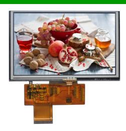
Sizes range from 3.5" to 7.0" with brightness ranging from 600~1000 cd/m2.
