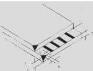
Corner chipping (ITO pins position)        | X                                                                                                                                                                                                                        | /                      | ≤1/6L        | /       |     | √   |
