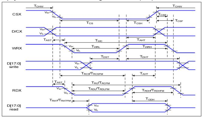
Figure 1 Parallel Interface Timing Characteristics (8080-Series MCU Interface)
