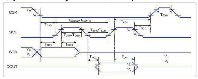
Figure 4 3-line serial Interface Timing Characteristics
