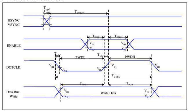
Figure 6 RGB Interface Timing Characteristics
