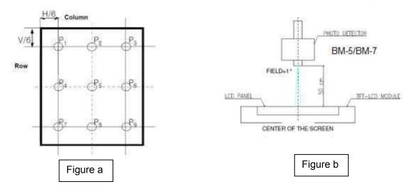
FIG.3. The definition of viewing angle
