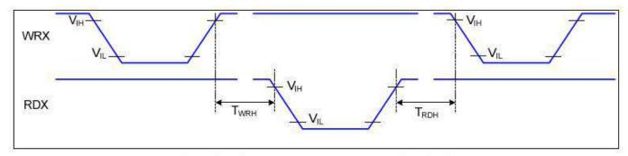
Figure 3 Write-to-Read and Read-to-Write Timing
