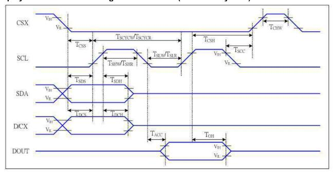
Figure 5 4-line serial Interface Timing Characteristics
