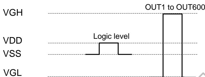
The logic levels of CPV, L/R, OE1, OE2, OE3, /XAO, MODE1, MODE2, SEG1, SEG2, EVEN, STV1 and STV2 have to swing between VDD for "H" and VSS for "L". PATH2 has ESD protection diodes connected to VDD and to VSS, the signal on PATH2 should also swing between VDD and VSS.
