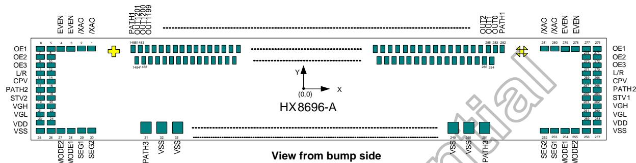
Chip size: 23650μm x 670μm (scribe line included)
