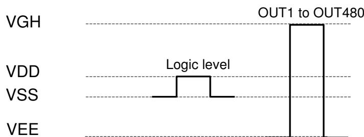
The logic levels of CPV, L/R, OE1, OE2, OE3, /XAO, MODE, STV1 and STV2 have to swing between VDD for "H" and VSS for "L".
