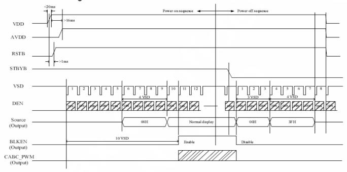
To prevent device latch up or power on display noise, the power on/off sequence shown below must be followed. After VDD reaches 1.8V, VGH/VGL can start to power on. Before VDD drops to 1.8V, VGH/VGL must start to power down. After VGH/VGL start to power on, CPV and STV should be not floating, and /XAO should be at VDD level or floating. The other control signals have no timing limitation.
