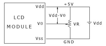
Vdd-V0: LCD Driving Voltage
