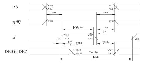
NOTE: \*VOL1 is assumed to be 0.8V at 2 MHZ operation.
