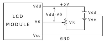
Vdd-V0: LCD Driving Voltage
