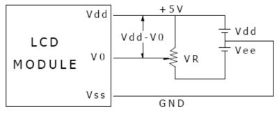
Vdd-V0: LCD Driving Voltage VR: 10K - 20K
