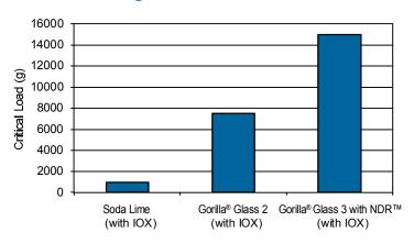
It takes more load to initiate radial cracks in the glass.
