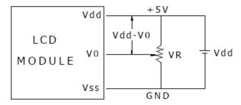
Vdd-V0: LCD Driving Voltage
