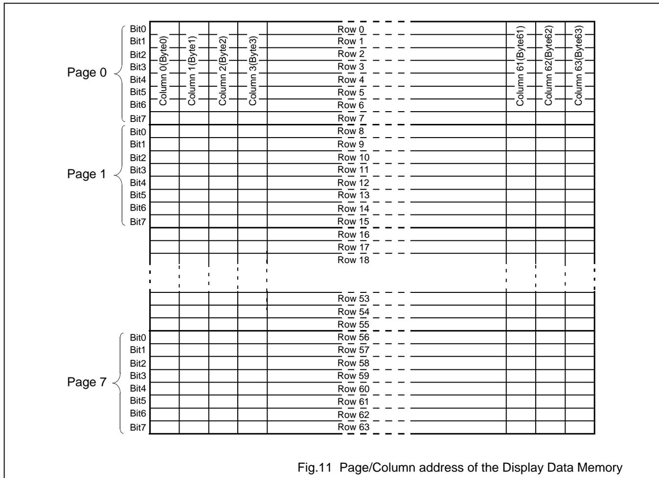
Fig.11 Page/Column address of the Display Data Memory
