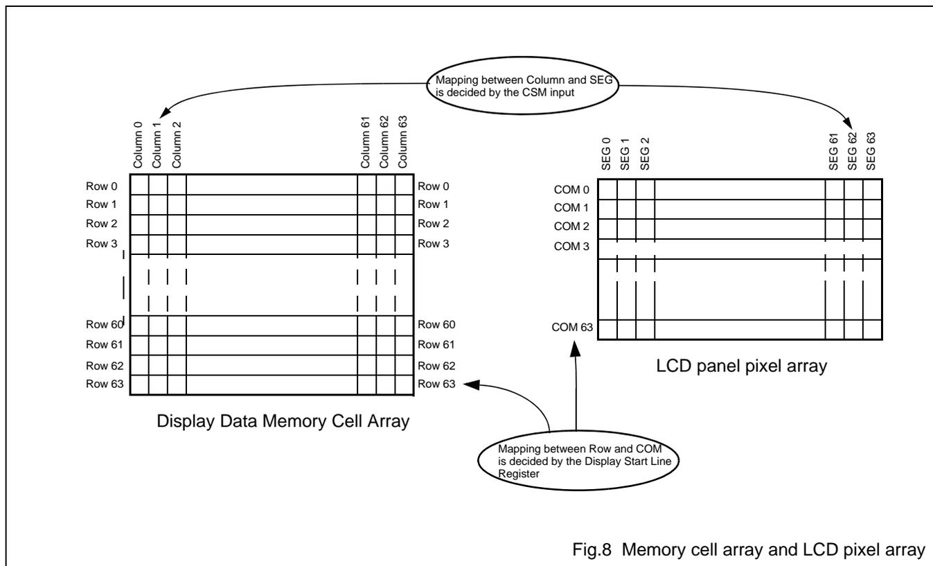
Fig.8 Memory cell array and LCD pixel array
