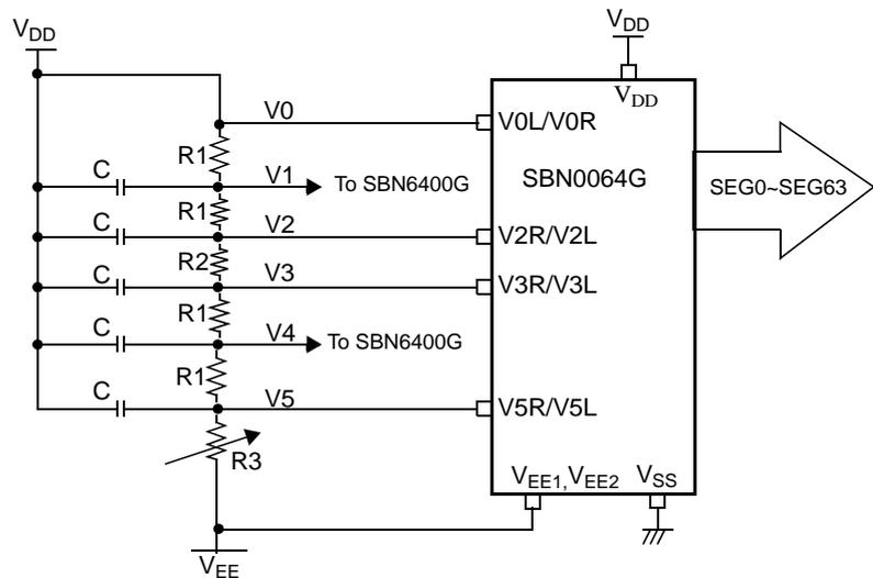
Fig.13 LCD Bias circuit
