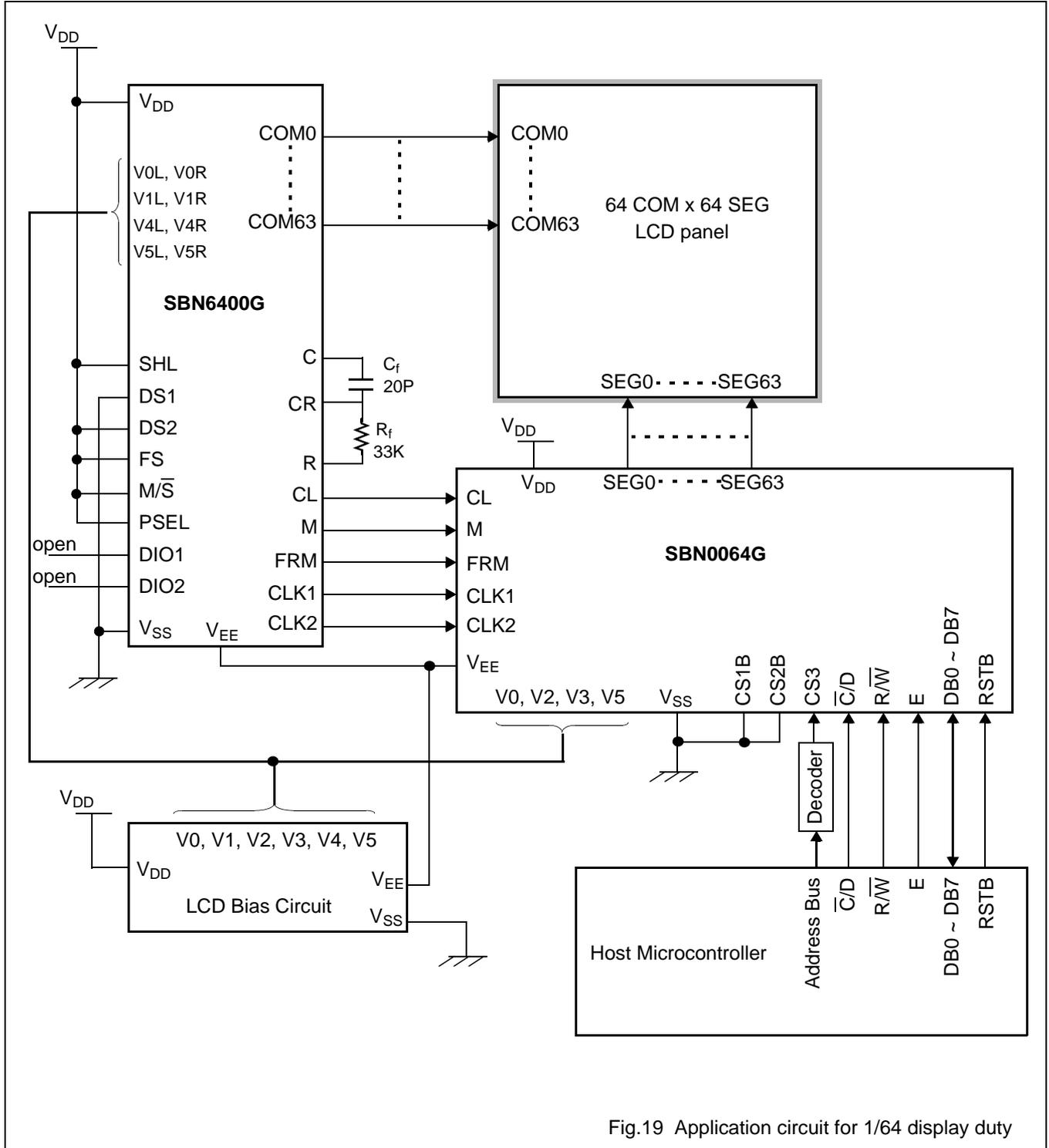
Fig.19 Application circuit for 1/64 display duty
