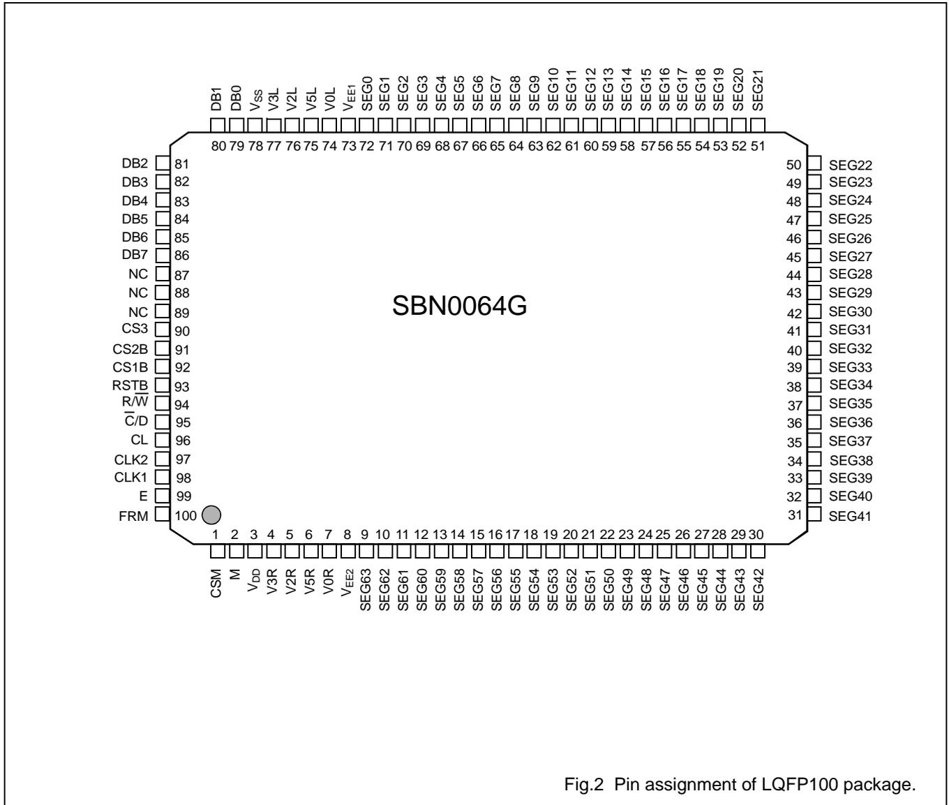
Fig.2 Pin assignment of LQFP100 package.
