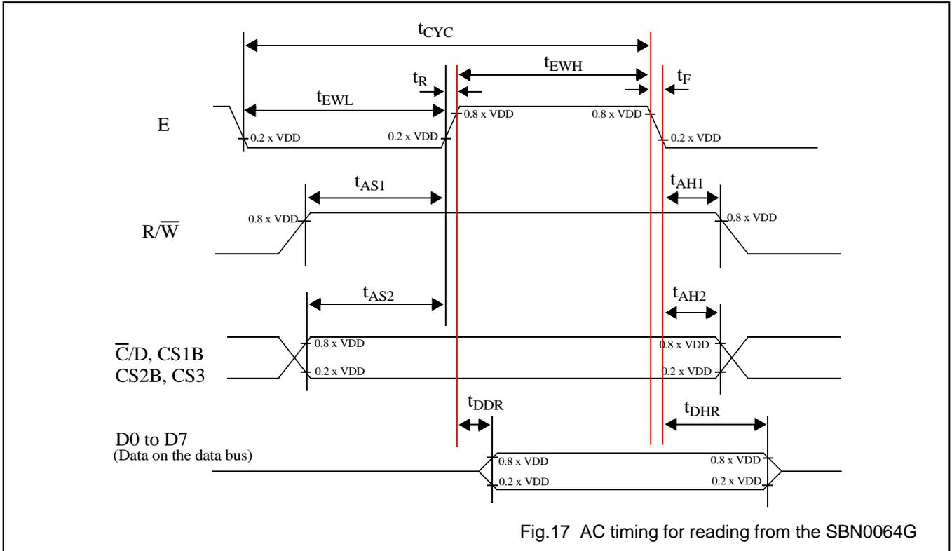
Fig.17 AC timing for reading from the SBN0064G
