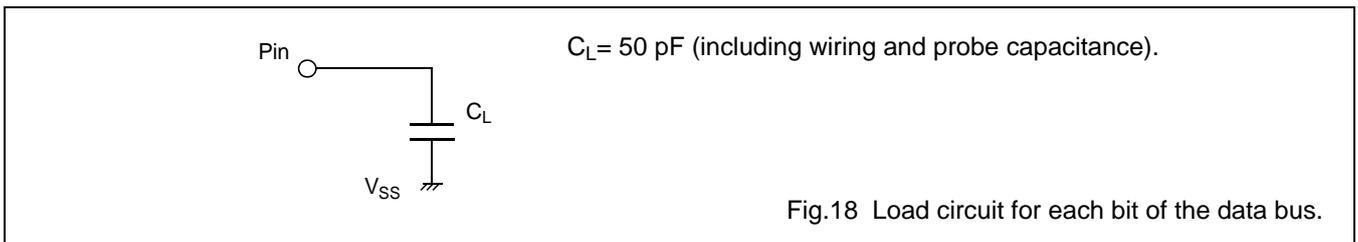
Fig.18 Load circuit for each bit of the data bus.
