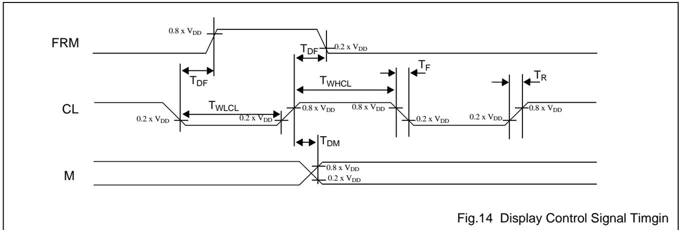
Fig.14 Display Control Signal Timgin
