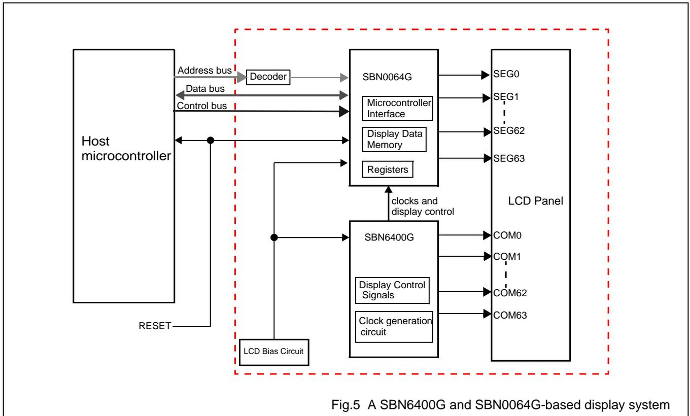
Fig.5 A SBN6400G and SBN0064G-based display system
