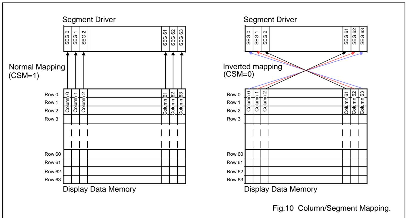
Fig.10 Column/Segment Mapping.
