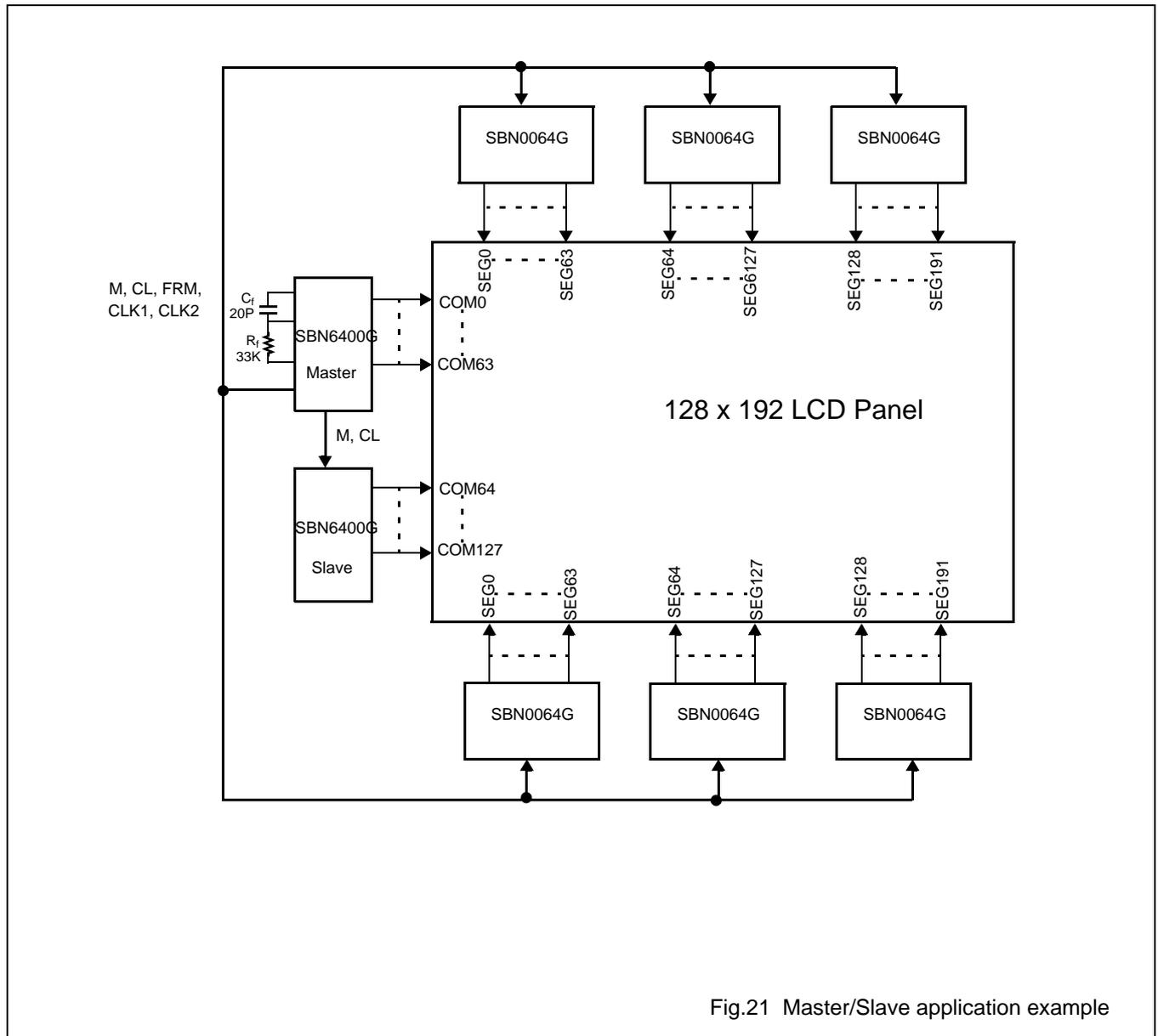
Fig.21 Master/Slave application example
