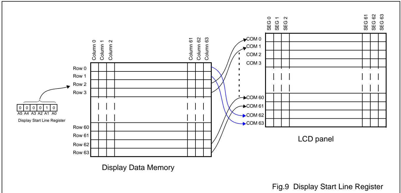
Fig.9 Display Start Line Register
