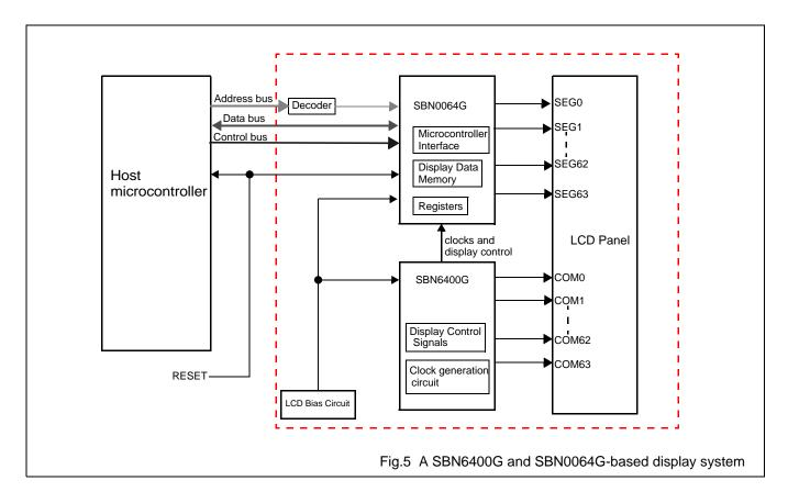
Dot-matrix STN LCD 64-SEGMENT Driver with 64-row x 64-column Display Data Memory
