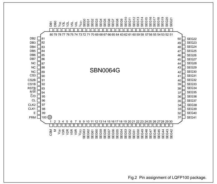
Dot-matrix STN LCD 64-SEGMENT Driver with 64-row x 64-column Display Data Memory
