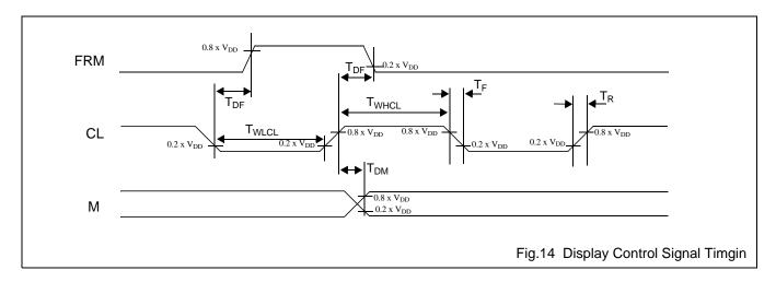
**Table 23** Display control signal (CL, FRM, and M) timing characteristics at  $V_{DD}$ =5 volts  $V_{DD}$  = 5 V ±10%;  $V_{SS}$  = 0 V; all voltages with respect to  $V_{SS}$  unless otherwise specified;  $T_{amb}$  = -20 to +75 °C.
