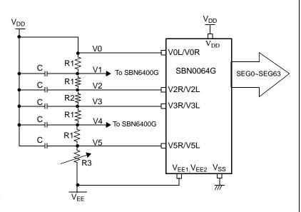
Fig.13 LCD Bias circuit
