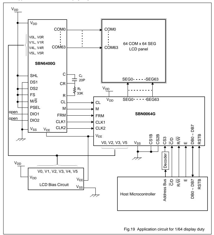
Dot-matrix STN LCD 64-SEGMENT Driver with 64-row x 64-column Display Data Memory
