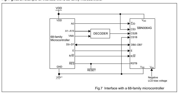
Dot-matrix STN LCD 64-SEGMENT Driver with 64-row x 64-column Display Data Memory
