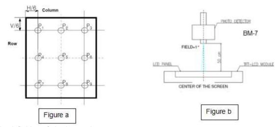
FIG.3. The definition of viewing angle
