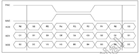
Figure 10.4: 6-bit LVDS input
