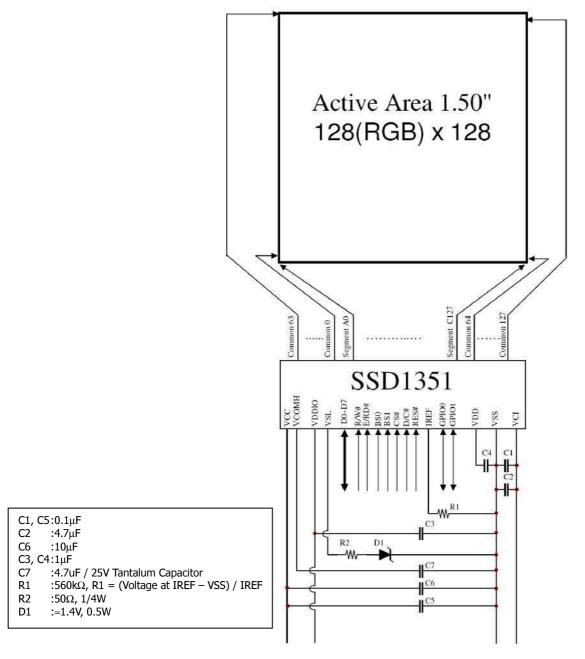
MCU Interface Selection : Base on BS0 and BS1 connection, showed as below table. Pins connected to MCU interface : D7~D0, E/RD#, R/W#, CS#, D/C#, and RES#
