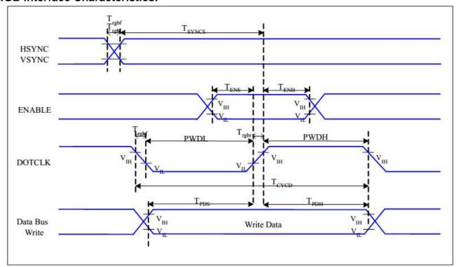
Figure 6 RGB Interface Timing Characteristics
