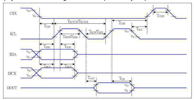
Figure 5 4-line serial Interface Timing Characteristics
