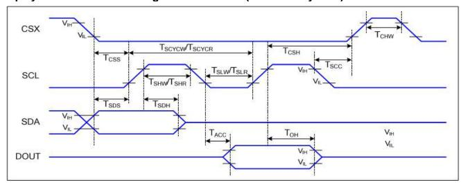
Figure 4 3-line serial Interface Timing Characteristics
