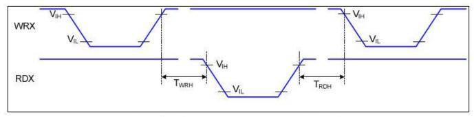
Figure 3 Write-to-Read and Read-to-Write Timing
