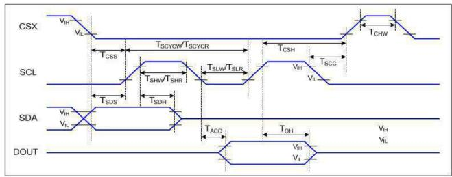
Figure 4 3-line serial Interface Timing Characteristics
