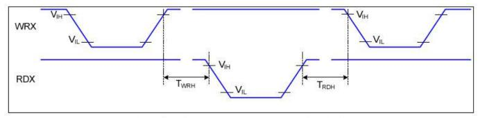
Figure 3 Write-to-Read and Read-to-Write Timing
