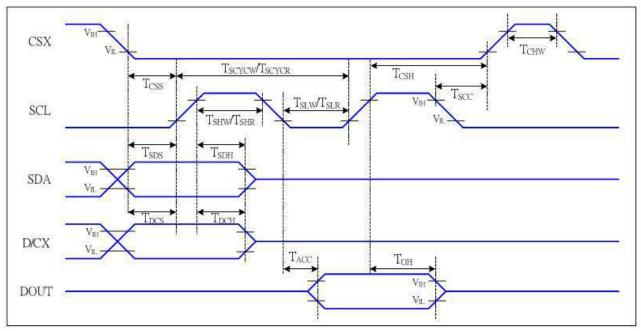
Figure 5 4-line serial Interface Timing Characteristics
