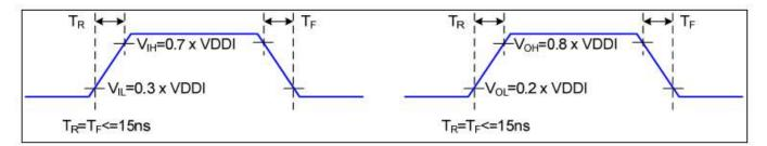
Figure 2 Rising and Falling Timing for I/O Signal
