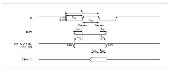
Figure 3. MPU Write Timing
