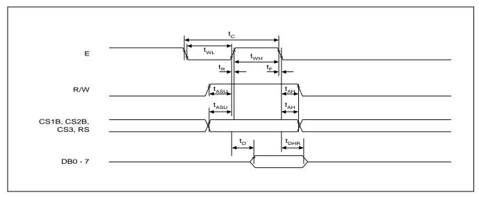
Figure 4. MPU Read Timing
