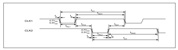
Figure 1. External Clock Waveform
