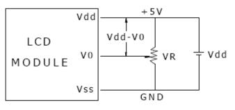
Vdd-V0: LCD Driving Voltage VR: 10K - 20K
