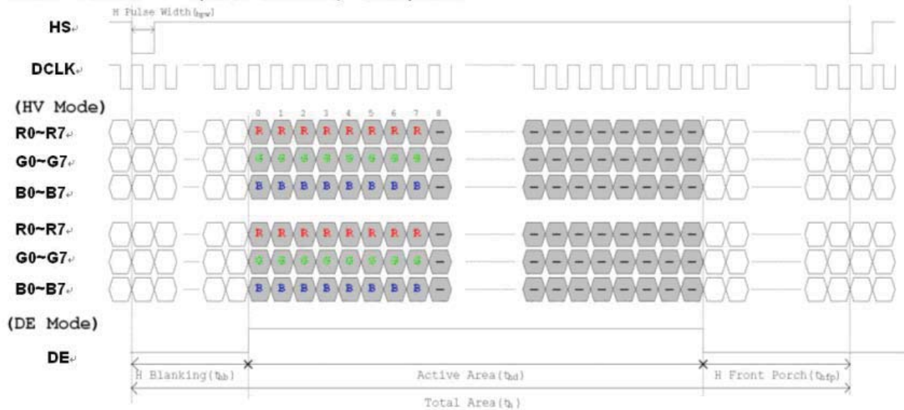
Horizontal input timing diagram.
