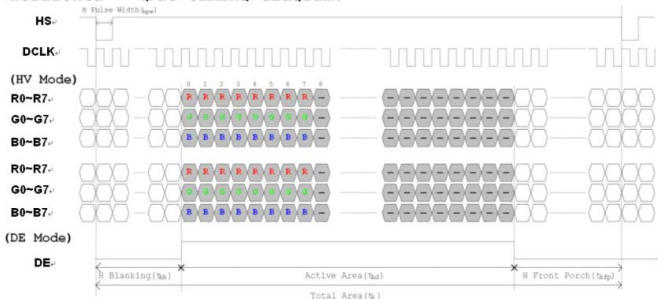
Horizontal input timing diagram.
